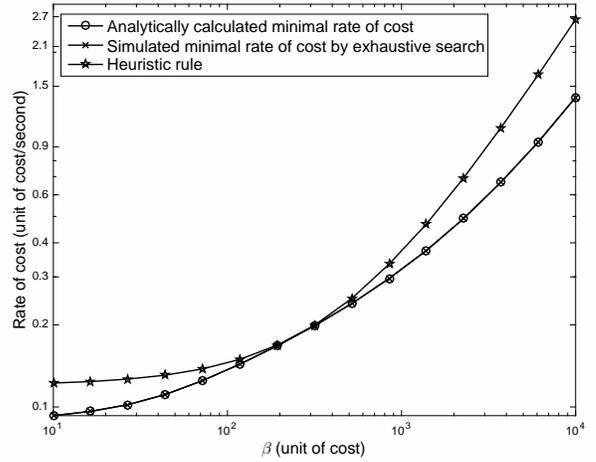
Fig. 3. The rate of cost in conditional pure-threshold strategies.
