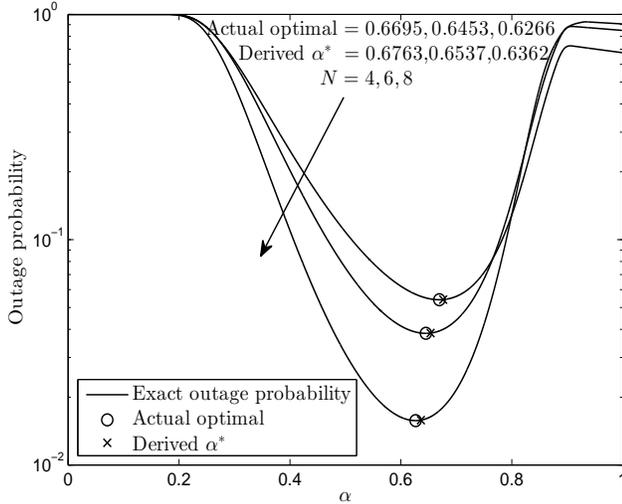
Fig. 3. Comparison of the derived time allocation factor  $\alpha^*$  with the actual optimal time allocation factor when the system SNR is  $\bar{\gamma} = 30$  dB.
