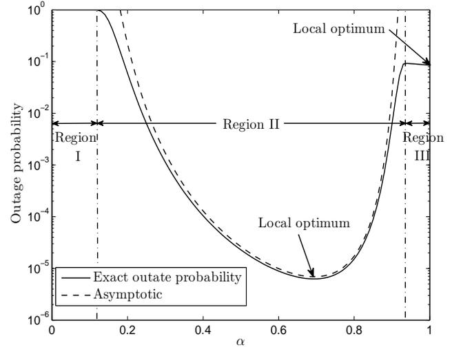
Fig. 2. The outage probability versus the time allocation factor  $\alpha$  with  $\eta = 2.6$ ,  $\mu = 1$ , and  $\bar{\gamma} = 30$  dB. Here the source is located at  $(0, 0)$ , and four users are randomly distributed within a circle centered at  $(3, 0)$  and with radius of 1 (specifically, the four users have randomly generated locations  $(3.5401, 0.0264)$ ,  $(3.3860, -0.4696)$ ,  $(2.9944, 0.3468)$ , and  $(3.0764, 0.7981)$ ).
