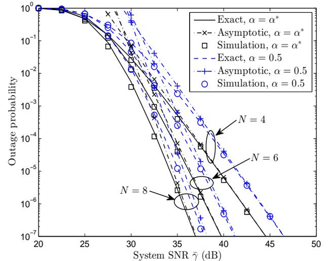
Fig. 6. Outage probability of the proposed scheme with the proposed time allocation and fixed time allocation ( $\alpha = 0.5$ ) in mixed Rayleigh/Rician fading channels, where the Rician  $K$ -factor is  $K = 5$  dB.
