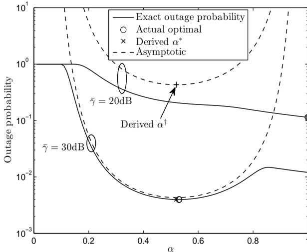
Fig. 4. Comparison of the derived time allocation factor  $\alpha^*$  with the actual optimal time allocation factor when there are only two users. Here the source is in the middle point of the two users, and the system SNR is  $\bar{\gamma} = 20$  dB or 30 dB.
