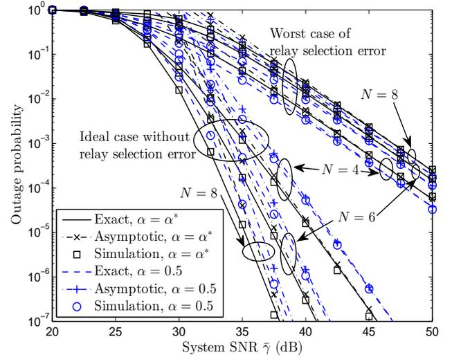
Fig. 5. Outage probability of the proposed scheme with the proposed time allocation and fixed time allocation ( $\alpha = 0.5$ ) when the channels follow Rayleigh fading.
