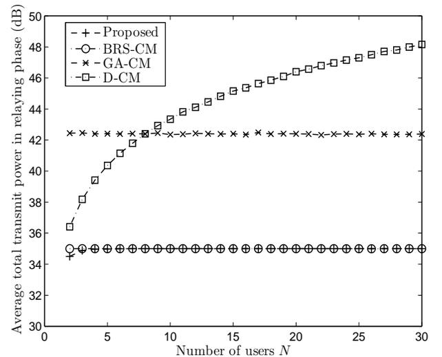
Fig. 8. Power consumption in the relaying phase of the proposed scheme, the D-CM scheme, the GA-CM scheme, and the BRS-CM scheme, with  $\bar{\gamma} = 35$  dB.
