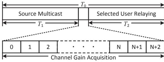
Fig. 1. Three portions for transmission of a multicast message.
