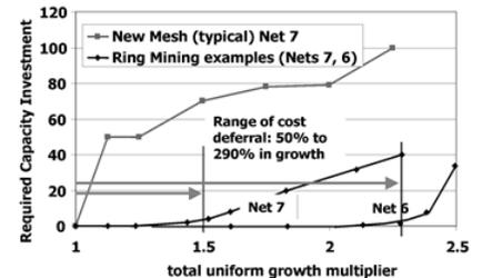
Figure 3: Typical Results of Ring Mining
