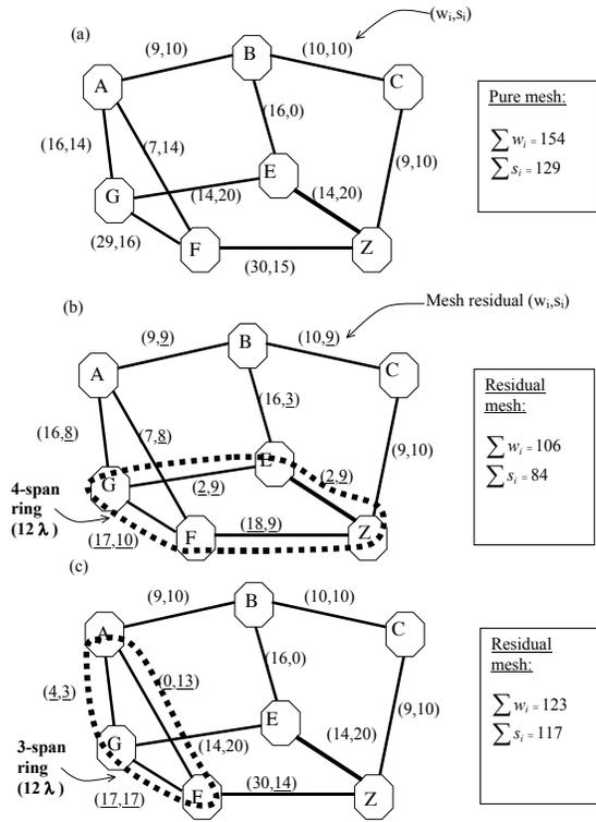
Figure 2(a) Optimized pure-mesh design, (b) ring with CRR = 0.97, (c) CRR=0.60
