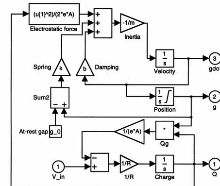
Figure 7.8. SIMULINK implementation of state equations for the parallel-plate electrostatic actuator. The labeling of the various blocks, including the use  $g_0$  to represent  $g_0$ , is characteristic of SIMULINK block diagrams.
