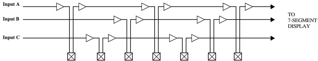
This test architecture allows us to test that all of the I/O pins are working, and that no solder bridges or other short-faults exist between any three adjacent I/O pins.
