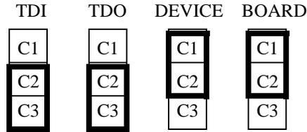
**FIGURE 2. Jumper Settings for Programming only the EPM7128S (MAX) Device**
