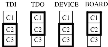
To run the UP1 board test, use the jumper settings shown in figure 3.
