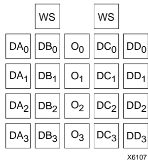
Figure 4-33 Rectangular Placement of RAM
