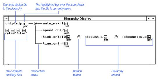
When you open the Hierarchy Display, it shows the full hierarchy of design files—called a "hierarchy tree"—for the current project or another hierarchy of design files. If one or more files in the hierarchy are open, the top of its file icon displays a highlighted bar. The Hierarchy Display shows the entire hierarchy of design files, as well as all user-editable ancillary files for the top-level design file, if the project has been compiled with the Compiler Netlist Extractor module.
