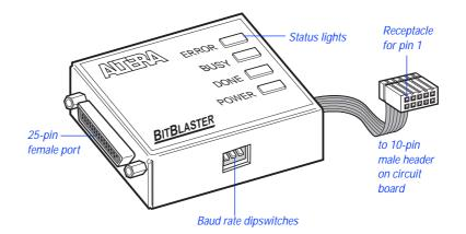
Figure 1-12. BitBlaster and 10-Pin Female Connector
