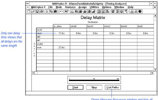
Opens Message Processor window and lists all delay times and paths between a pair of nodes.
