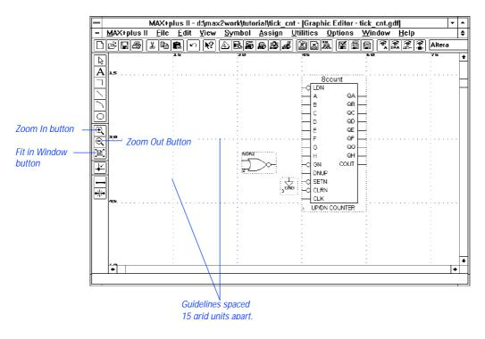
As you edit your schematic, you can change the window display to view larger or smaller portions of the file by choosing the **Zoom In**, **Zoom Out**, and **Fit in Window** buttons on the tool palette, as shown in the previous illustration.
