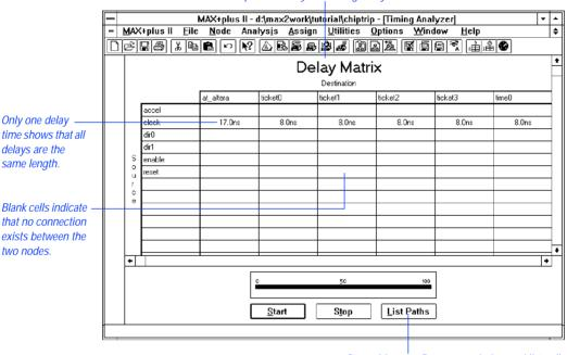
Delay Matrix is one of three types of analyses performed by the Timing Analyzer.
