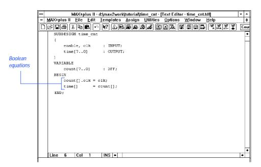
Once you have defined the group, square brackets ([]) are a shorthand way of specifying the entire range. The first equation connects the subdesign's clk input to the flipflops' Clock ports. The second equation sets the time[] inputs equal to the count[] variables.
