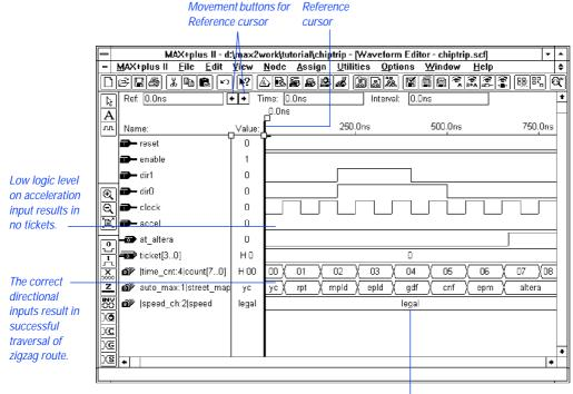
Low logic level on acceleration input is reflected in the "legal" state.
