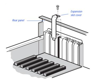
Figure 1-5. Removing the Expansion Slot Cover
