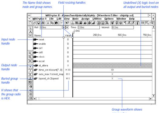
Figure 2-22. MAX+PLUS II Waveform Editor
