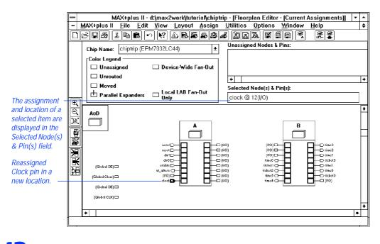
Go to "Back-Annotating Assignments for a Project" and "Finding Nodes & Pins in the Floorplan Editor" using **Search for Help on** (Help menu) for more information on using the Floorplan Editor.
