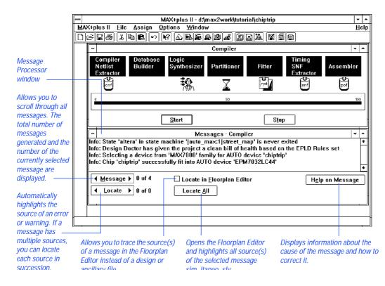
As shown in the illustration, the Design Doctor has given the **chiptrip** project a "clean bill of health," and the Compiler has selected the EPM7032LC44 device (an EPM7032 device in a 44-pin plastic J-lead chip carrier package) for the project.
