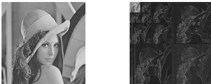
Figure 8. Wavelet Forward Transform Example (3 levels decomposition)
