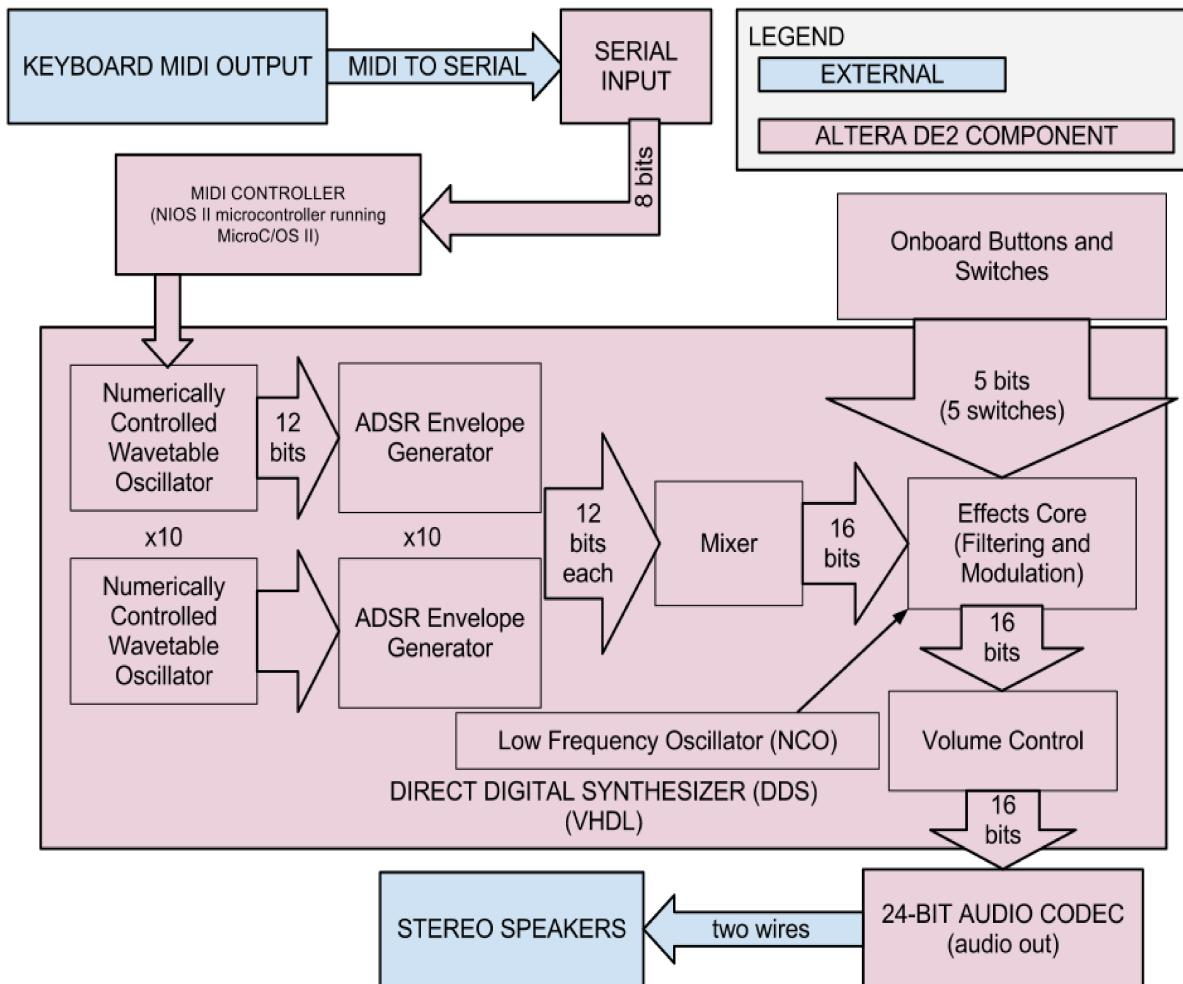
A typical synthesizer unit is made up of the following elements, all of which will be implemented on the Altera DE2 FPGA:
