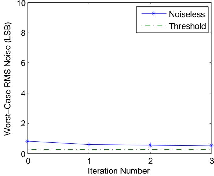
Figure 3.5: RMS noise of noiseless tone mapping versus number of iterations. Ideally, the RMS noise should be below the visibility threshold but it is close enough, even with zero iterations.
