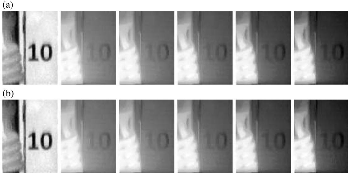
Figure 4.9: Corresponding frames of a video after (a) floating-point operation in Matlab and (b) fixed-point operation in C (real time). There is an abrupt DR change happening when the bulb is turned on. The difference between (a) and (b) is difficult to detect by eye. Although the frame interval is 20 ms, every tenth frame is shown over a 1 s period.
