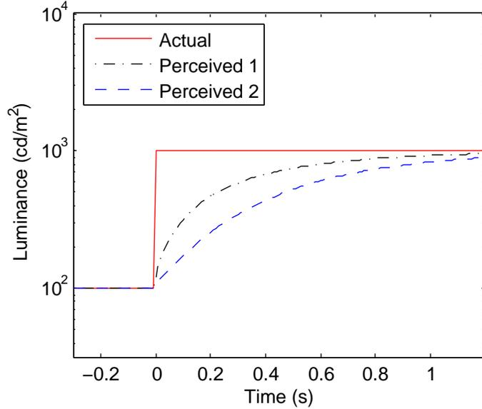
Figure 3.8: The process of temporal adaptation during luminance change. The Perceived 1 curve applied a LPF to luminance while a LPF is applied to brightness for the Perceived 2 curve. Both perceived luminances model temporal adaptation but the latter is easier to compute.
