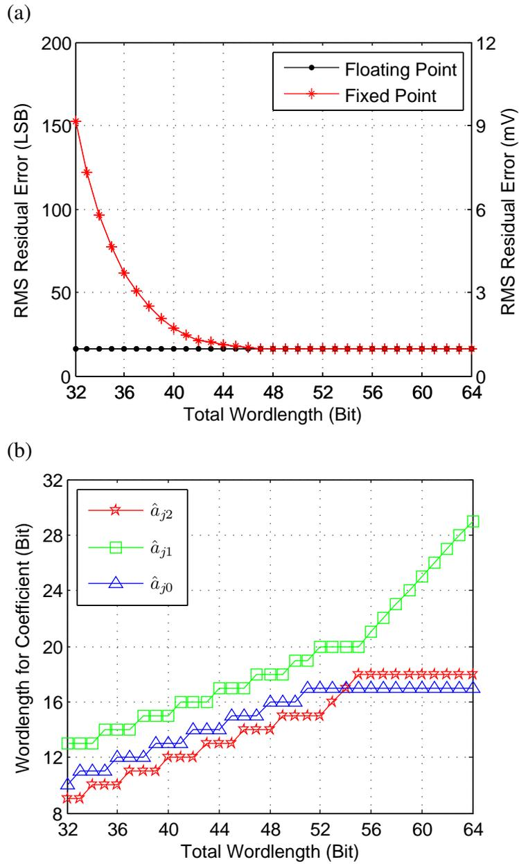
Figure 4.6: (a) RMS residual error is represented in two ways: digital response (left Y axis) and voltage (right Y axis). (b) Optimal wordlength distribution for coefficients, which is decided by minimizing RMS residual error for each total wordlength.
