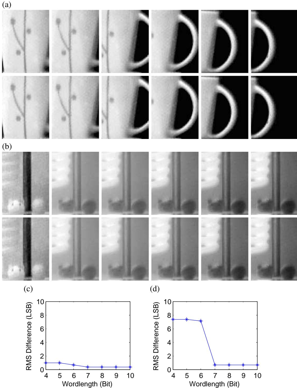
Figure 4.8: Frames in two sequences show (a) motion and (b) an abrupt DR change (when the bulb is turned on). The top frames use floating-point noiseless tone mapping (with temporal adaptation) while the bottom frames use the fixed-point design. RMS differences of sequences (a) and (b) are shown in (c) and (d) under different wordlengths for LPF coefficients. Although there are 200 frames over a 4 s period, every tenth frame is shown over a 1 s period.
