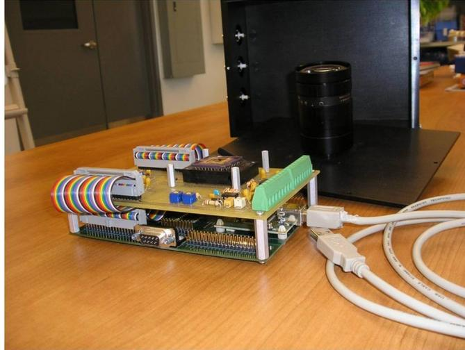
Figure 1.3: Prototype of a digital camera with a logarithmic CMOS image sensor. The PCB board and QuickUSB board are connected by a ribbon cable. The boards are put inside the camera body. (This picture was taken by Orit Skorka.)
