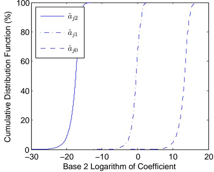
Figure 4.1: After FPN calibration, the magnitude distribution of each coefficient across pixels indicates a need for different scale factors. Using the same scale factor for each coefficient may result in saturation, depending on wordlength.
