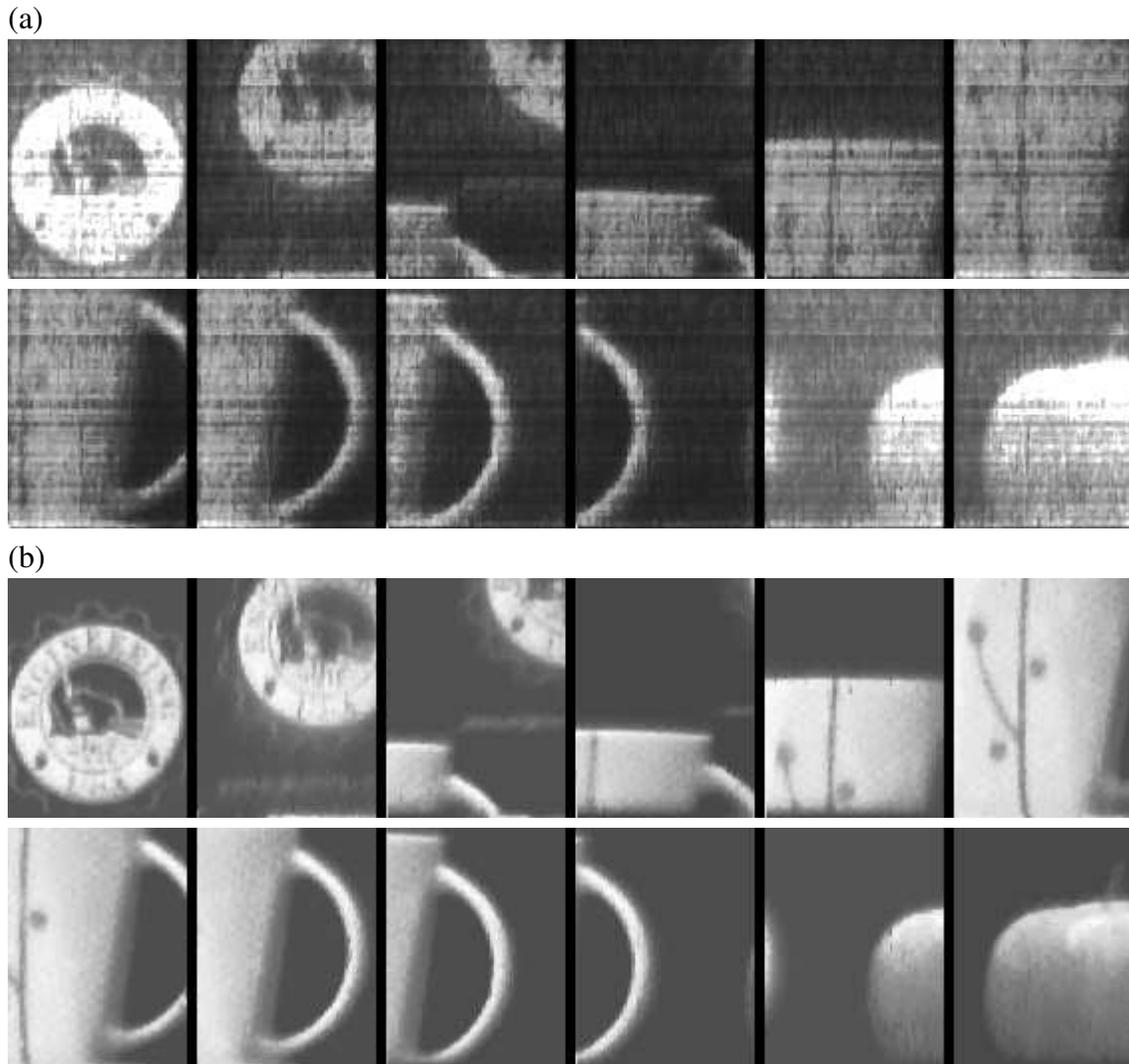
Figure 2.5: Video of a scene (a) before and (b) after three-parameter IPR FPN correction. These examples demonstrate the suitability of the method for real-time processing. Although the frame interval is 20 ms, every tenth frame is shown to highlight dynamics.
