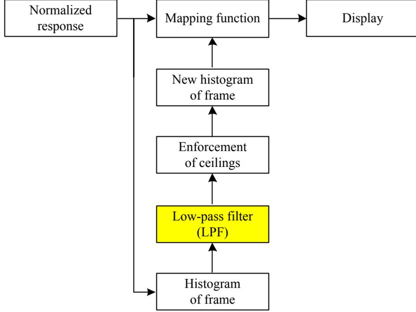
Figure 3.7: Flow chart of noiseless tone mapping. The highlighted block is added for noiseless tone mapping with temporal adaptation. Ceilings are calculated once beforehand. The mapping function is built from the new histogram.
