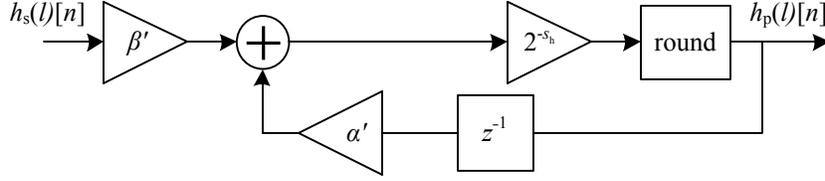
Figure 4.5: Fixed-point first-order low-pass filter, which is used for noiseless tone mapping with temporal adaptation. Filter coefficients are first scaled and then stored in fixed-point format. Finally, the result is scaled back.
