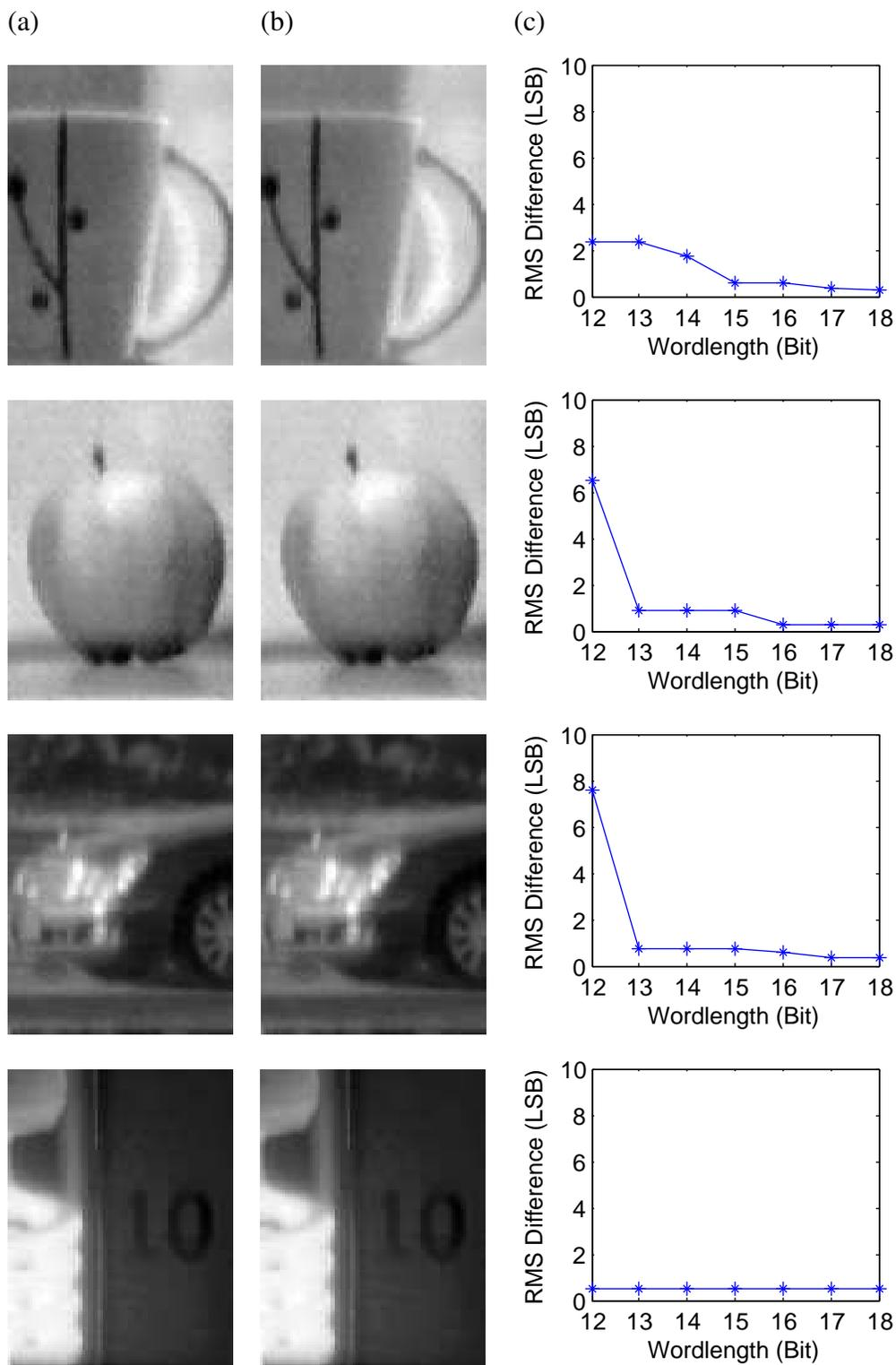
Figure 4.7: Images after (a) tone mapping by floating-point operation and (b) tone mapping by fixed-point operation (optimal design). (c) RMS difference versus parameter wordlength. Visual differences are quantified on the right. The RMS difference reduces with wordlength increase. Differences are difficult to see when the images are mapped by the optimal fixed-point design.
