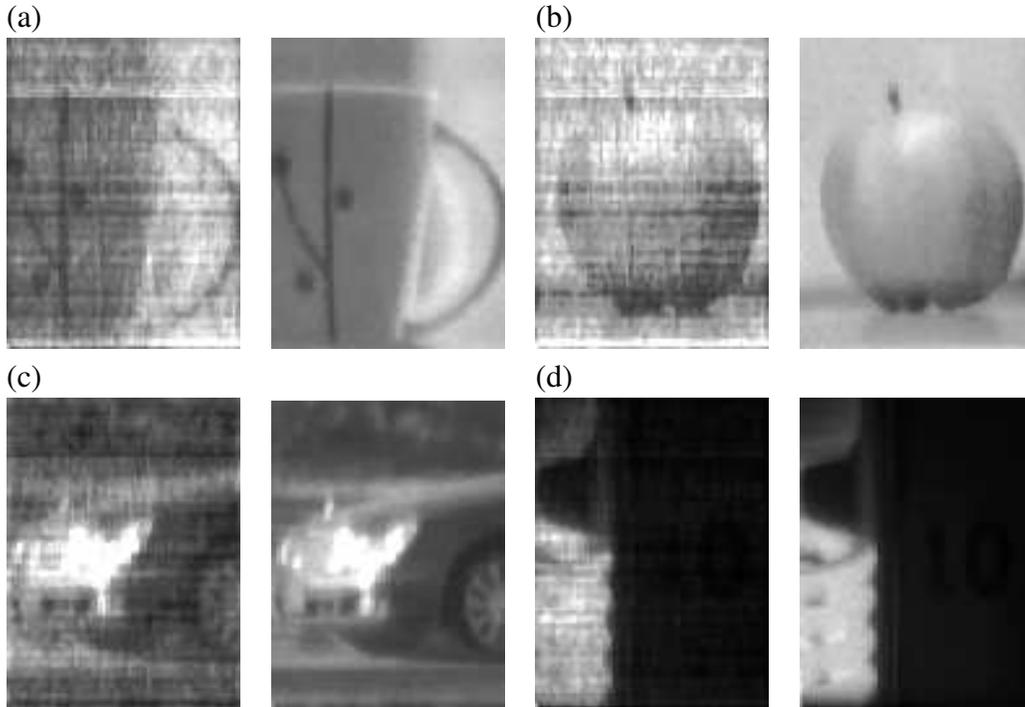
Figure 2.4: Original image (left) and image after three-parameter IPR FPN correction (right) for four scenes. The proposed correction reduces FPN effectively, which improves the image quality. Simple tone mapping makes it difficult to render high-DR scenes for a standard display. In (c), the headlight of the car is overexposed. In (d), the dark part of the scene is underexposed. Nevertheless, FPN is corrected.
