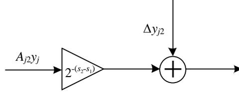
Figure 4.4: The model for first-level dynamic shifting can be represented as follows: the result of multiplication is scaled and then added to round-off error, which is introduced by a truncation operation.
