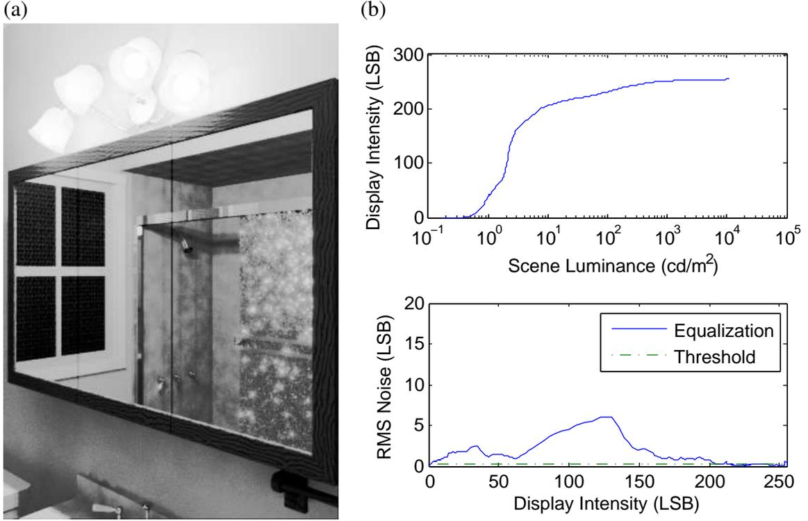
Figure 3.4: (a) Bathroom image with simulated camera noise after histogram equalization. (b) The mapping function (top) and displayed RMS noise (bottom). Camera noise is visible on the wall below the mirror.
