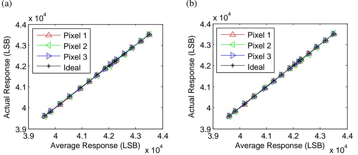
Figure 2.1: Three-parameter (a) PR and (b) IPR FPN correction of three pixels. The actual (corrected) responses of both methods approximate the average (ideal) response of all 10 800 pixels very well in a dynamic range of 5.3 to 33 000 cd/m<sup>2</sup>.
