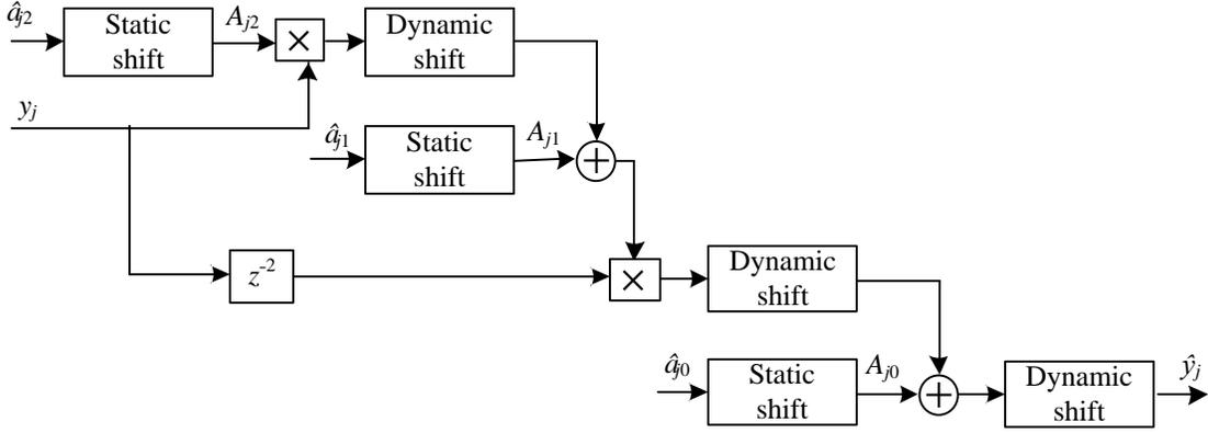
Figure 4.2: In this fixed-point design, static and dynamic shifting will introduce round-off errors. The total fixed-point error is the output-referred sum of round-off errors. We need to minimize it based on performance demands and wordlength limits.
