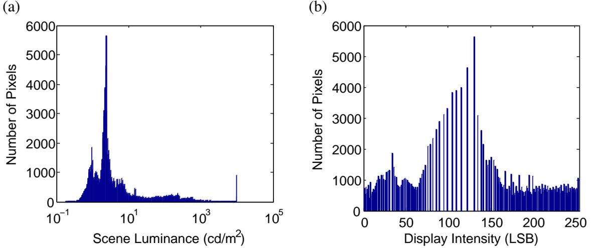
Figure 3.2: Histogram of the bathroom image. (a) The original histogram is not uniform. (b) After histogram equalization, pixel intensities are distributed more uniformly. Gaps in the new histogram occur because equalization is done on discrete data.
