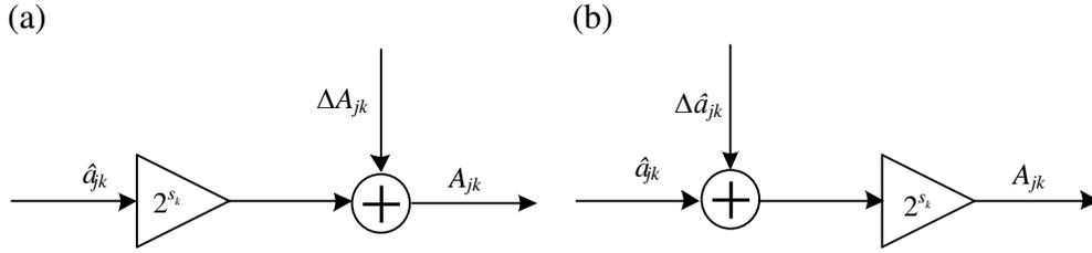
Figure 4.3: Coefficient scaling and rounding may be modeled in two ways: (a) original coefficient is scaled and static round-off error is added; or (b) original coefficient is added to unscaled static round-off error and the sum is then scaled.
