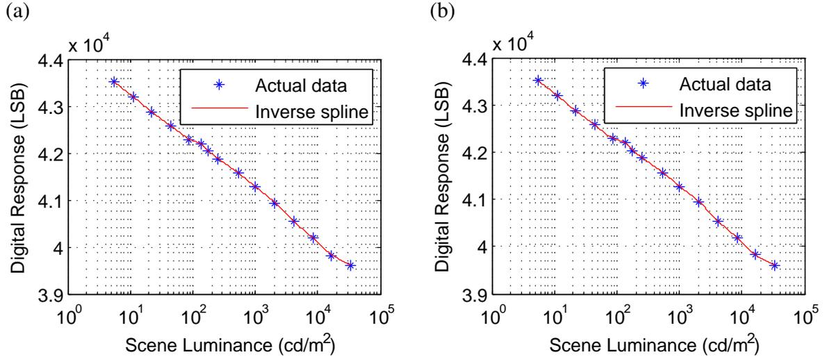
Figure 2.3: Response linearization based on (a) linear interpolation and (b) piecewise cubic Hermite spline interpolation using the calibration data. The difference between them is not obvious because of the log-scale X axis.
