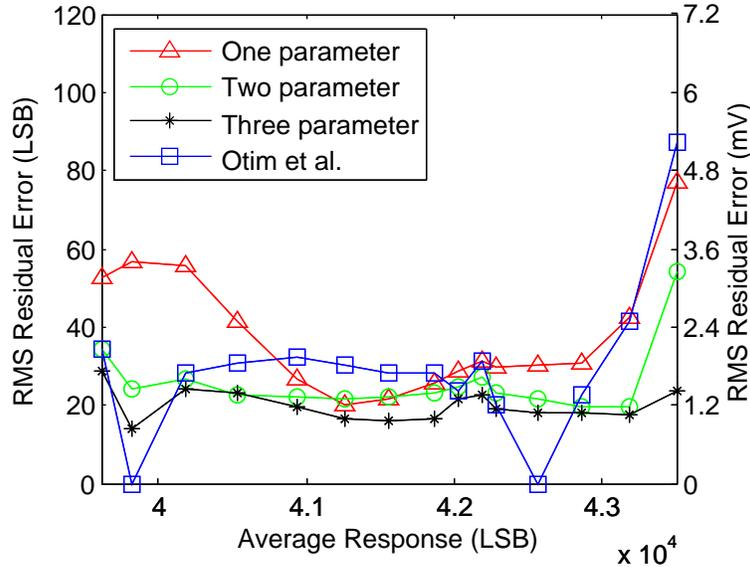
Figure 2.2: RMS residual error of various FPN correction methods, including one from Otim *et al.*'s FPN correction [21]. Three-parameter IPR correction provides the best performance among these corrections, considering all luminance levels.
