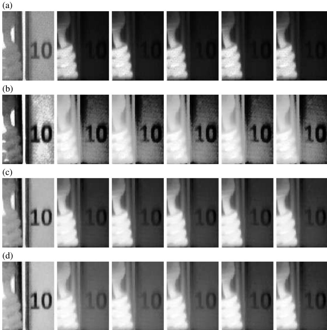
Figure 3.10: Video of scene changed from low DR to high DR. At left, a bulb is turned on while a printed “10” is on the right shielded by a separator. From (a) to (d) respectively, we use simple tone mapping, histogram equalization, noiseless tone mapping without temporal adaptation, and noiseless tone mapping with temporal adaptation. Although the frame rate is 45 Hz, every ninth frame over a 1 s period is shown for brevity.
