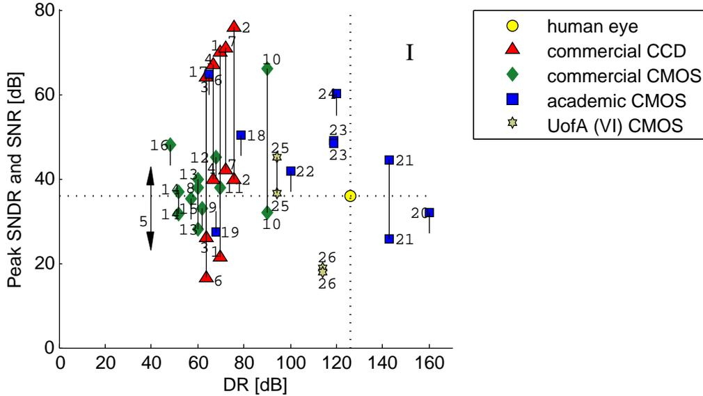
Figure 1.1: Linear sensors offer high SNR or SNDR while logarithmic sensors offer high DR. Sensors 25 and 26 are logarithmic CMOS DPS and logarithmic VI-CMOS APS prototypes, respectively, that were designed and tested at the University of Alberta. Logarithmic response offers high DR while pixel-level ADCs and nonlinear FPN correction provide high SNDR. The figure is provided by Skorka [1], incorporating data by Mahmoodi [16] and methods developed in this thesis.
