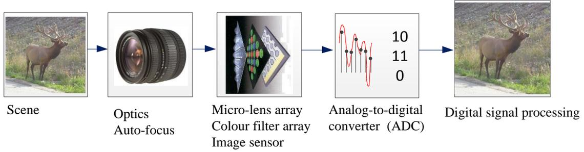
Figure 1.2: The components of a digital camera comprise mainly a lens, a color filter, an image sensor, one or more ADCs, and DSP. The ADCs in CMOS digital camera may be at chip level, column level, or pixel level. The work in this thesis focuses on the DSP part. (This figure was created by Orit Skorka and modified by Jing Li.)
