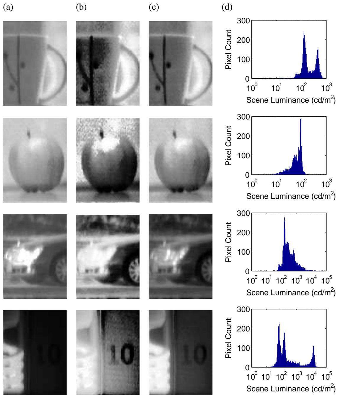
Figure 3.9: Low-DR (top two) and high-DR (bottom two) images after (a) simple tone mapping, (b) histogram equalization, and (c) noiseless tone mapping, respectively. Scene histograms, based on the original images, are given in (d).
