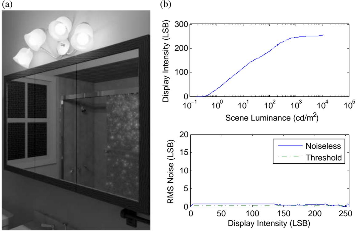
Figure 3.6: (a) Bathroom image with simulated camera noise after noiseless tone mapping. (b) The mapping function (top) and displayed RMS noise (bottom). Camera noise is invisible on the wall below the mirror.
