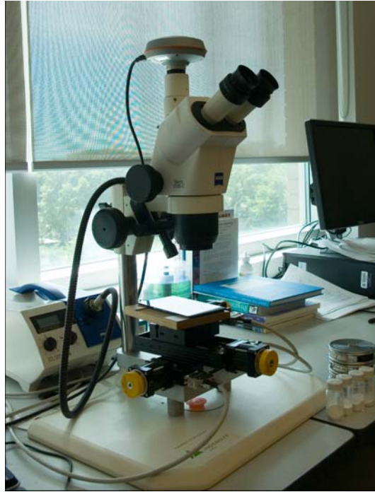
Figure 3.2: Computer-aided identification system setup. This picture illustrates the setup used in the computer-aided classification system of this thesis. Included in this setup is a microscope, motorized stage, custom stand, light source, digital camera, and sieving tools.
