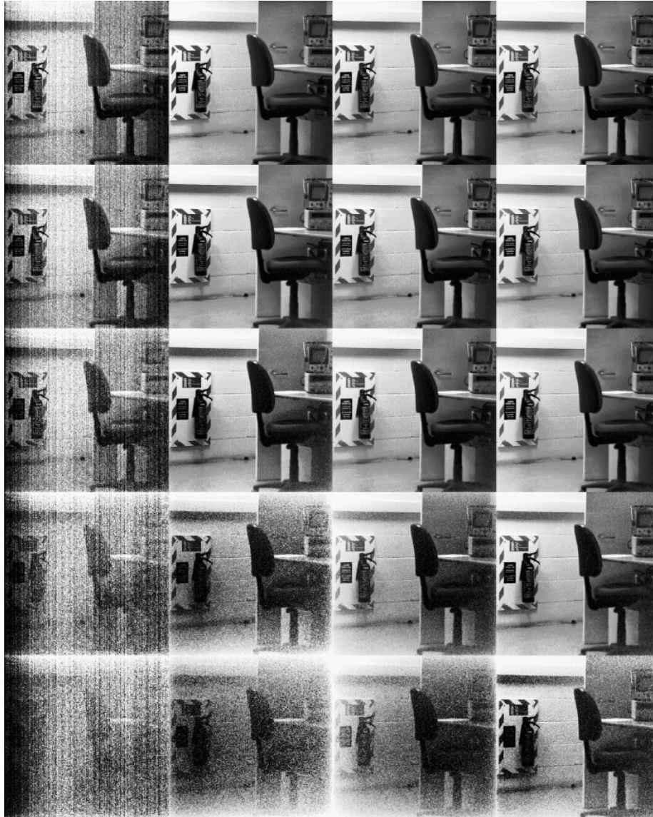
Figure 4.5: FPN correction of Fuga 15RGB images for the nil, single, double and triple variation models (left to right). The images, displayed in greyscale with histogram equalisation, are of one scene with illuminances attenuated by 0, 13, 21, 32 and 40dB (top to bottom) using neutral density filters over the camera lens.
