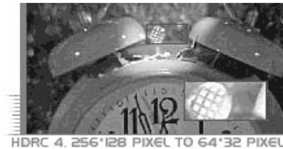
Figure 1.6: Since logarithmic pixels operate continuously, they permit high speed imaging especially when frame size is traded for frame rate. In this example from IMS Chips, the subframe rate of 4000Hz is 16 times faster than the full frame rate [4].
