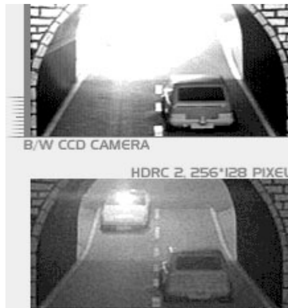
Figure 1.5: An image from IMS Chips shows how linear cameras (CCD or CMOS) saturate when they encounter a high dynamic range scene whereas logarithmic cameras (CMOS only) capture perceptible detail in the bright and dark parts of the scene [4].
