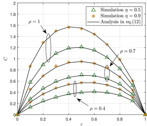
Fig. 4. Average throughput of delay-tolerant mode versus  $\tau$  for  $P = 1$  dBm and  $N = 3$ .
