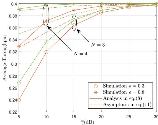
Fig. 2. Average throughput of delay-limited mode versus SNR  $\bar{\gamma}$  for  $\tau = 0.6$ ,  $\eta = 0.7$  and  $R = 1$ .
