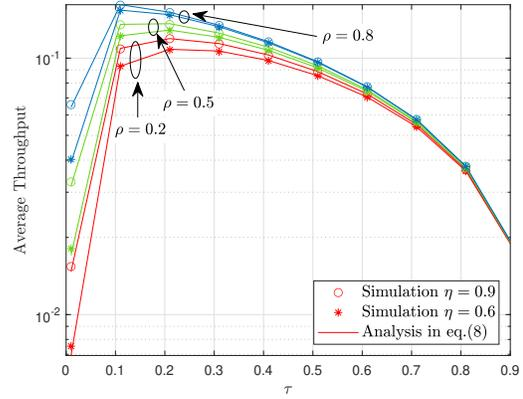
Fig. 3. Average throughput of delay-limited mode versus  $\tau$  for  $N = 3$ ,  $P = 10$  dBm.
