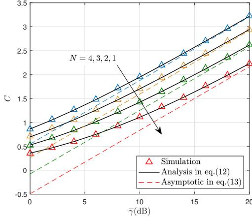
Fig. 5. Average throughput of delay-tolerant mode versus SNR  $\bar{\gamma}$  for  $\eta = 0.9$ ,  $\tau = 0.6$ ,  $\rho = 0.6$ .
