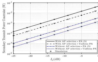
Fig. 2(b): Transmit power constraint versus  $I_p$ . The curves are generated using analysis and simulation.
