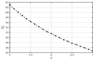
Fig. 2(a): The number of active secondary APs  $M_0^s$  versus  $\delta$ . The curve is generated analytically, not via simulations.
