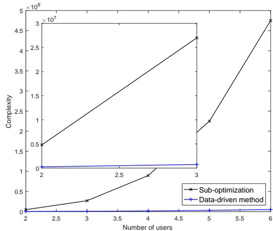
Fig. 8. Complexity of sub-optimization and data-driven method
