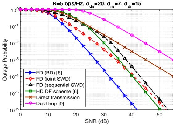
Fig. 5. Comparison between the outage probabilities of FD DF relaying with BD and SWD, HD DF relaying [6], dual-hop [9] and direct transmissions.
