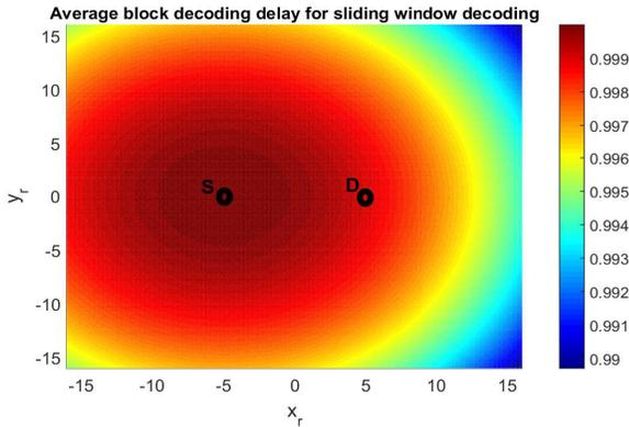
Fig. 3. Average block decoding delay of FD DF relaying with SWD for any  $\mathcal{R}$  location in  $2D$  plan where  $B = 1000$ .
