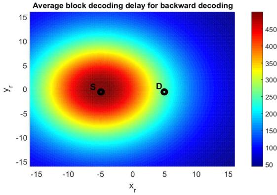
Fig. 2. Average block decoding delay of FD DF relaying with BD for any  $\mathcal{R}$  location in  $2D$  plan where  $B = 1000$ .
