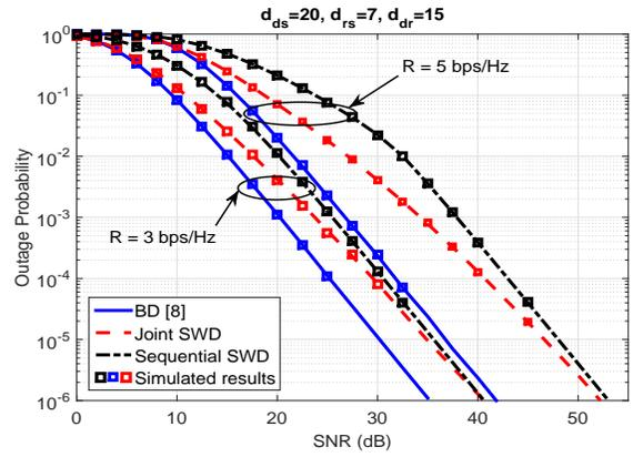
Fig. 4. Outage probabilities of FD DF relaying with BD, joint and sequential SWD at different target rates  $R$ .
