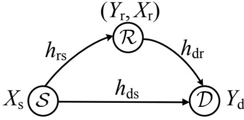
Fig. 1. Basic Relay channel model.
