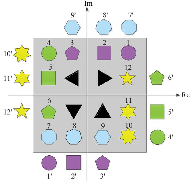
Fig. 1. The cyclically extended 16-QAM constellation diagram.
