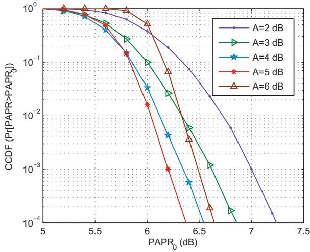
Fig. 5. CCDFs of different PAPR thresholds of CN-TI scheme with eight iterations, 16QAM, and 256 subcarriers.
