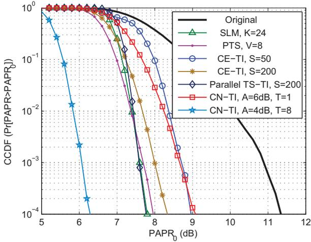
Fig. 2. CCDFs of the PAPR for various schemes with 128 subcarriers.
