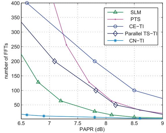
Fig. 4. PAPR vs. computational complexity comparison of the various schemes with 256 subcarriers.
