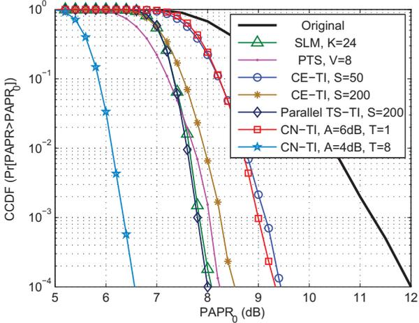
Fig. 3. CCDFs of the PAPR for various schemes with 256 subcarriers.
