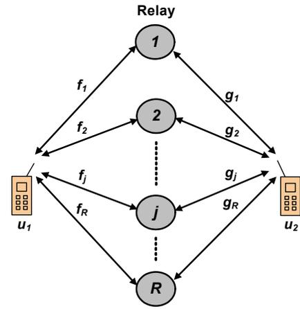
Fig. 1. A two-way multiple-relay network with two end users and  $R$  relays.
