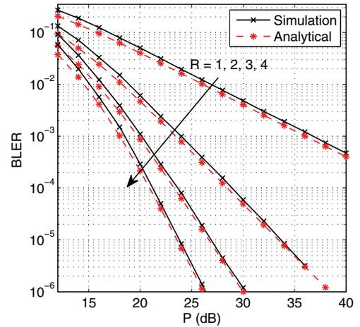
Fig. 4. BLER of the SRS scheme ( $R = 1, 2, 3, 4$  and  $P = Q_j$ ).
