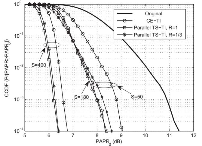
Fig. 2. CCDFs of the PAPR for various TI schemes with 128 subcarriers.
