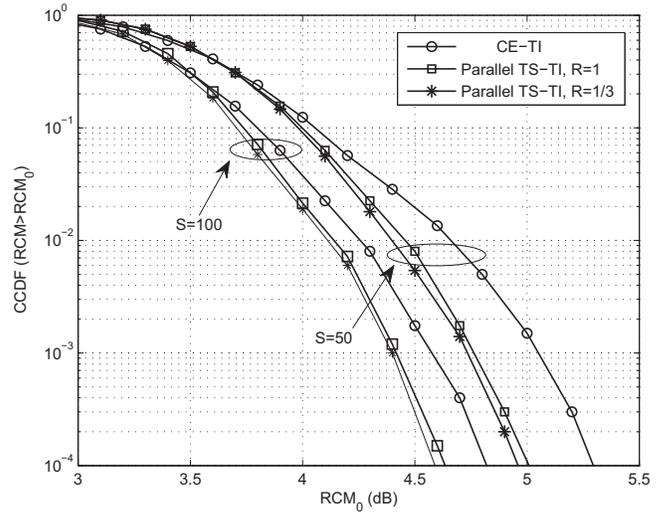
Fig. 7. CCDFs of the raw cubic metric comparison of the CE-TI and Parallel TS-TI schemes.
