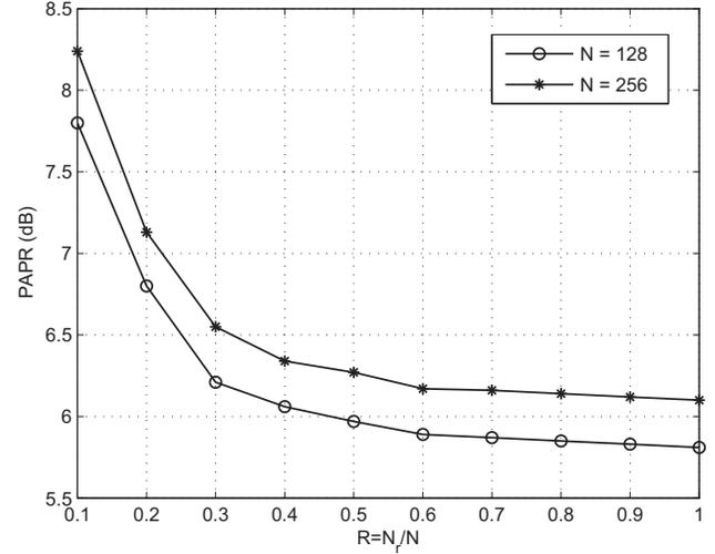
Fig. 6. PAPR reduction vs. proposed parameter  $R$  in the Parallel TS-TI scheme.
