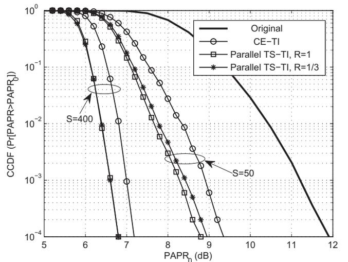
Fig. 3. CCDFs of the PAPR for various TI schemes with 256 subcarriers.
