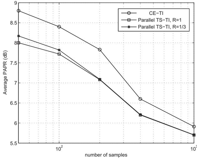
Fig. 4. Average PAPR reduction comparison of the CE-TI and Parallel TS-TI schemes for the same complexity.
