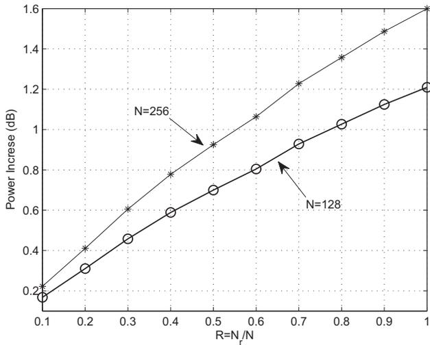
Fig. 5. Power increase vs. proposed parameter  $R$  in the Parallel TS-TI scheme with the 6 dB PAPR threshold.
