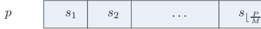
(b) A generic symbol, s_j , and a transmitted packet, p , which is formed by defined symbols
