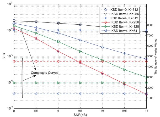
Fig. 3. Comparison of the IKSD and conventional KSD for a coded  $4 \times 4$  MIMO 16-QAM system.
