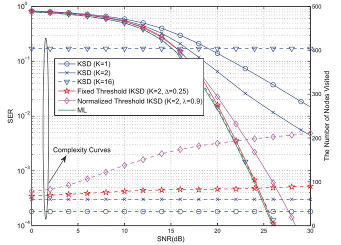
Fig. 1. Comparison of the IKSD and KSD for an uncoded  $4 \times 4$  MIMO 16-QAM system.
