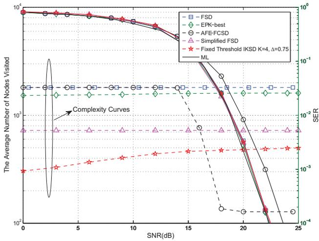
Fig. 2. Comparison of different SD algorithms for an uncoded  $8 \times 8$  MIMO 16-QAM system.
