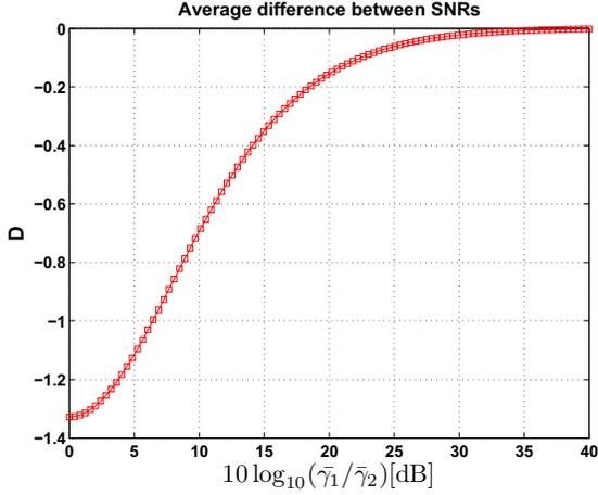
Fig. 5. Average difference between the actual SNR and the approximate SNR obtained by HMA (see Eq. (18)) as a function of mean SNR ratio.
