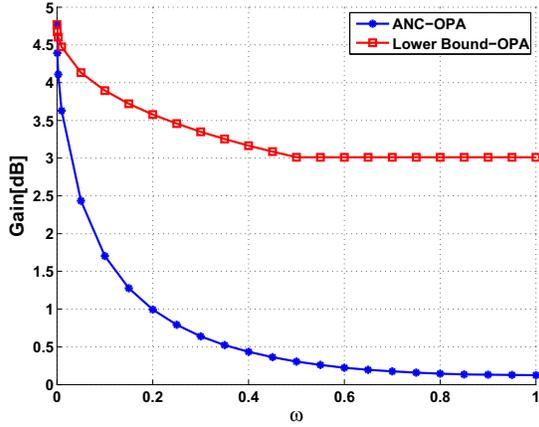
Fig. 3. Power allocation gain with respect to ANC with a fixed target rate.
