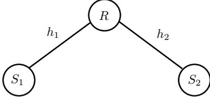
Fig. 1. Two-way relay channel (TWRC) model.
