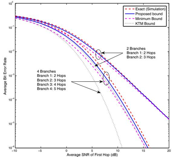
Fig. 4. The BPSK average BER bounds of multi-hop multi-branch relay network with MRC at the destination. System operates over i.i.d. Rayleigh fading channels.  $P_l = \lfloor \frac{N_l}{2} \rfloor$ .
