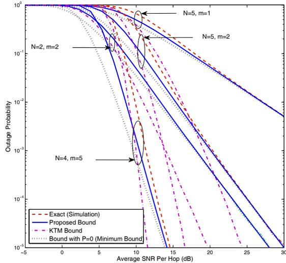
Fig. 2. A comparison of outage probability bounds of multi-hop relay network over i.i.d. Nakagami- $m$  fading channels.  $P = \lfloor \frac{N}{2} \rfloor$ .
