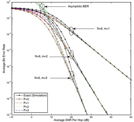
Fig. 3. The effect of  $P$ , number of hops and severity of fading on proposed BER bounds of a multi-hop relay network in i.i.d. Nakagami- $m$  fading.
