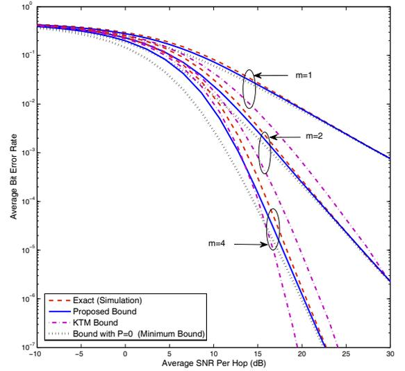
Fig. 1. A comparison of the effect of severity of fading on average BER bounds for a multi-hop relay network in i.i.d. Nakagami- $m$  fading.  $N = 3$  and  $P = 2$ .
