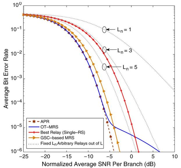
Fig. 4. Comparison of the average BER of BPSK of several RS schemes for a ten-relay cooperative network. The GSC-based MRS scheme selects the best five relays out of ten available relays.  $L = 10$ .
