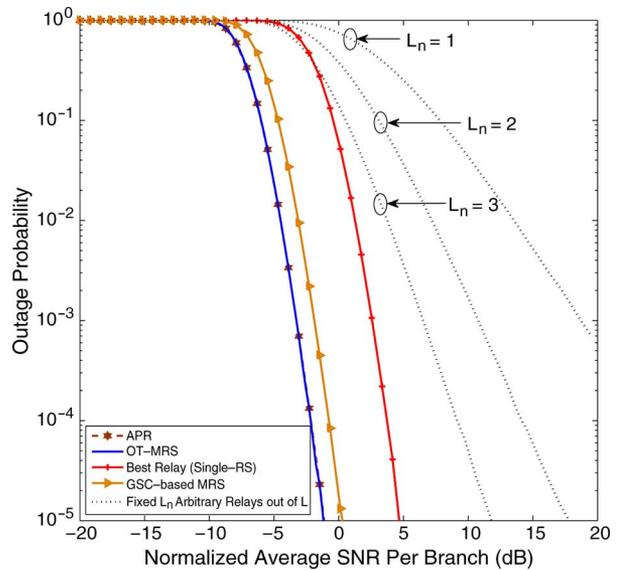
Fig. 5. Comparison of the SNR outage probability of several RS schemes. The GSC-based MRS scheme selects the best five relays out of ten available relays.  $\bar{\gamma}^* = \bar{\gamma}/\gamma_{th}$ .  $L = 10$ .
