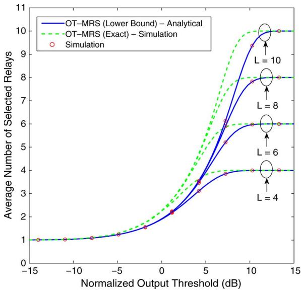
Fig. 3. Average number of selected relays  $\bar{L}_c$  versus normalized output threshold  $\bar{\gamma}_{th}^* = \gamma_{th}/\bar{\gamma}$ .
