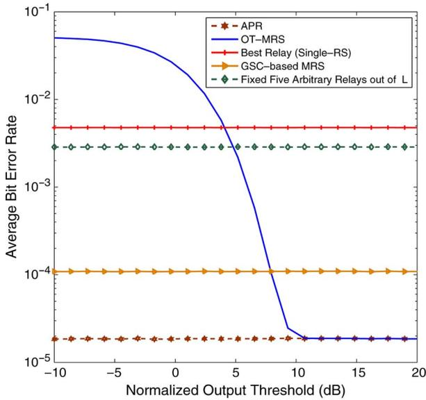
Fig. 6. Comparison of the BPSK BER of several RS schemes against the normalized output threshold  $\bar{\gamma}_{th}^*$ . The GSC-based MRS scheme selects the best five relays out of ten available relays.  $\bar{\gamma}_{th}^* = \gamma_{th}/\bar{\gamma}$ .  $\bar{\gamma} = 3$  dB.  $L = 10$ .
