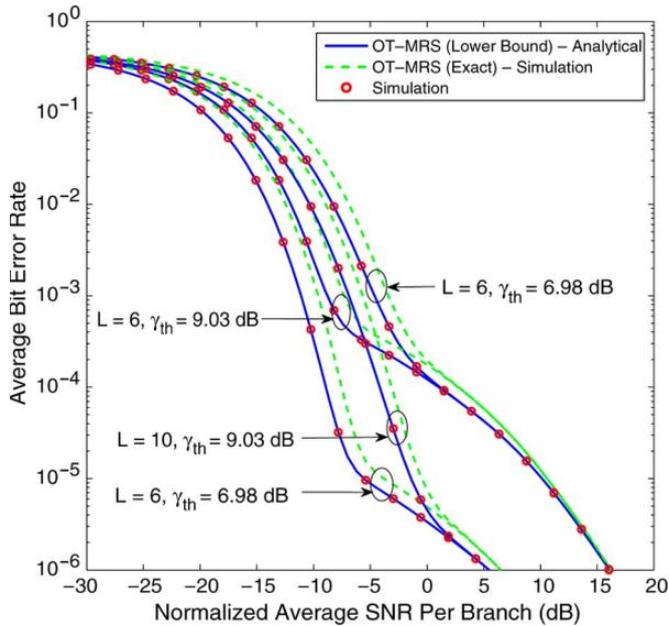
Fig. 2. Average BER of BPSK as a function of the normalized average SNR per branch ( $\bar{\gamma}^* = \bar{\gamma}/\gamma_{th}$ ).
