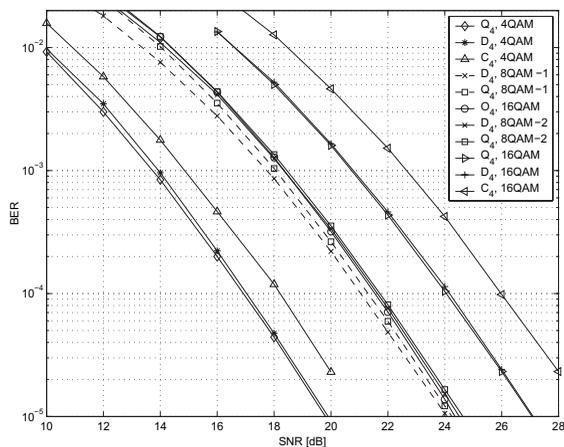
Fig. 2. Performance of MDC-ABBA codes for 4 Tx antennas compared with ABBA codes and OSTBC.
