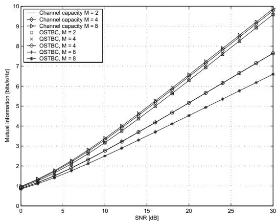
Fig. 1. MMI of ABBA/MDC-ABBA codes and OSTBC over MISO channels.
