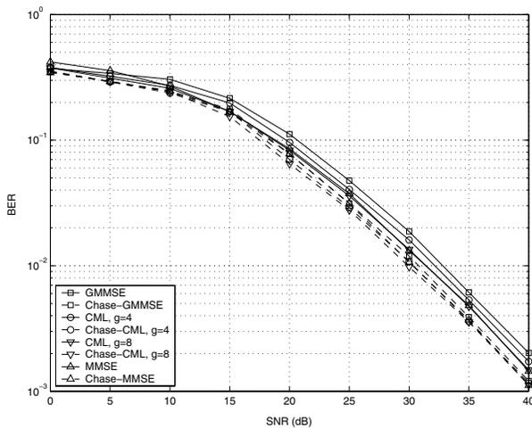
Fig. 2. Performance comparison of constrained linear detectors in an  $8 \times 8$  MIMO system with 16QAM.
