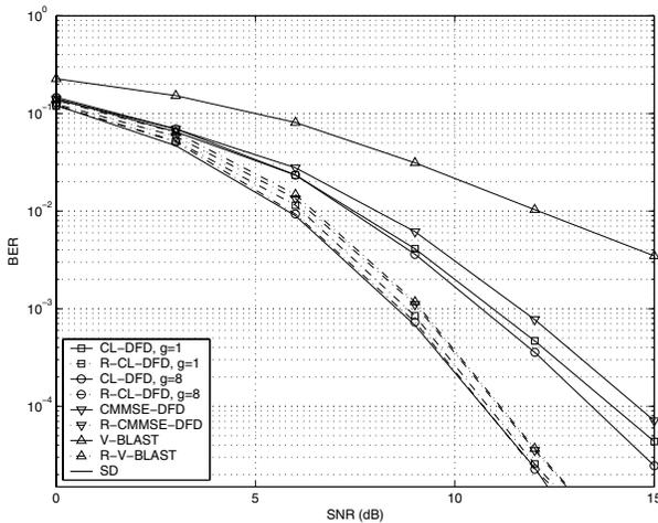
Fig. 3. Performance comparison of combined linear and decision feedback detectors in an  $8 \times 8$  BPSK MIMO system.
