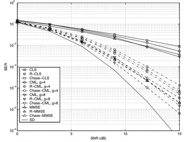
Fig. 1. Performance comparison of constrained linear detectors in an  $8 \times 8$  MIMO system with BPSK.
