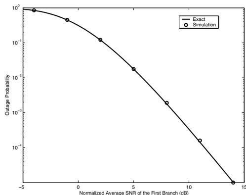
Fig. 1. Outage probability  $P_{out}$  of 4-branch SC versus the normalized average SNR of the first branch  $\bar{\gamma}_1/\gamma_{th}$  over correlated Rayleigh fading channel.
