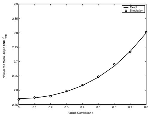
Fig. 2. The average output SNR of 3-branch EGC normalized by the first branch SNR.
