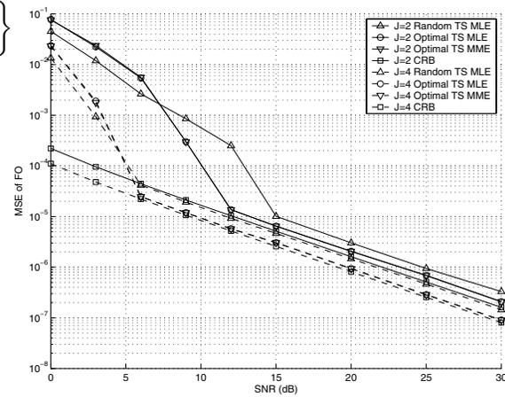
Fig. 1. The MSE of FO versus SNR with different  $J$  in a SISO channel
