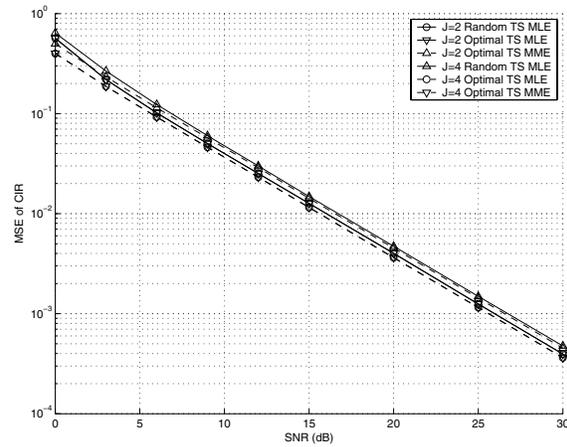
Fig. 5. The MSE of CIR versus SNR with different  $J$  in a MIMO channel
