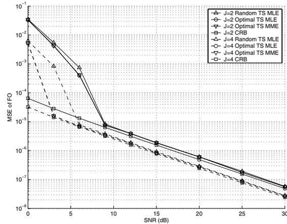
Fig. 4. The MSE of FO versus SNR with different  $J$  in a MIMO channel
