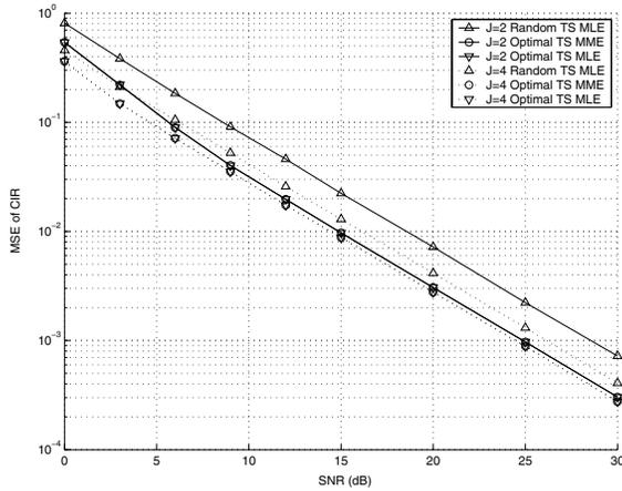
Fig. 2. The MSE of CIR versus SNR with different  $J$  in a SISO channel
