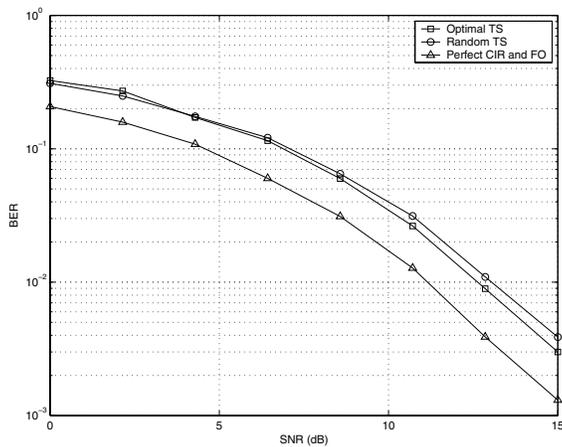
Fig. 3. BER versus SNR with randomly selected TS and optimal TS in a SISO channel
