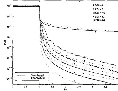
Fig. 2. Power spectral density of an OFDM signal with different number of carrier
