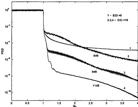
Fig. 5. Power spectral density of an OFDM signal passing through a SSPA with different IBOs (EGI=0,16).
