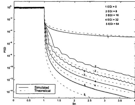
Fig. 3. Power spectral density of an OFDM signal with an extended guard interval.
