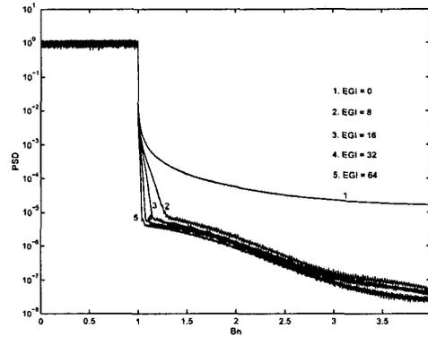
Fig. 7. Power spectral density of an OFDM signal with different EGIs passing through a SL (IBO=9dB).
