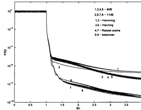
Fig. 11. A comparison of OBR with different windowing functions(EGI=16).
