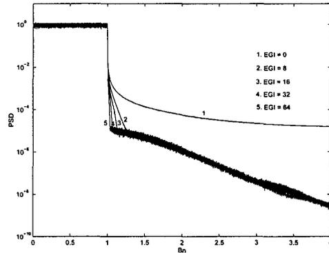
Fig. 8. Power spectral density of an OFDM signal with different EGIs passing through a SSPA (IBO=9dB).
