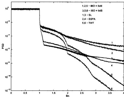
Fig. 10. A comparison of OBR of an OFDM signal with different nonlinearities (EGI=16).
