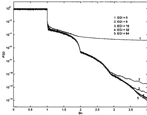
Fig. 9. Power spectral density of an OFDM signal with different EGIs passing through a TWT (IBO=9dB).
