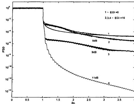
Fig. 4. Power spectral density of an OFDM signal passing through a SL with different IBOs (EGI=0,16).
