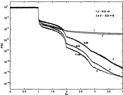
Fig. 6. Power spectral density of an OFDM signal passing through a TWT with different IBOs (EGI=0,16).
