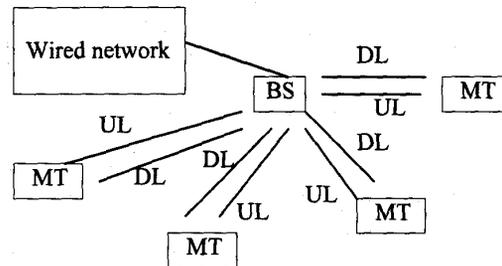
Figure 1 A BS-MT system (cell) in a wireless packet network
