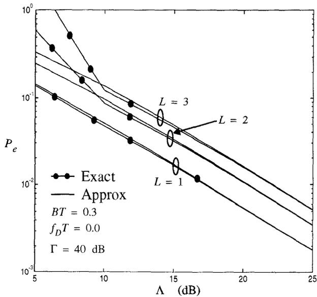
FIGURE 2. The exact and approximate bit error rates of GMSK in a Rayleigh fading environment in the presence of  $L$  cochannel interferers, The detection method is LDD. Infinite CDR is assumed.
