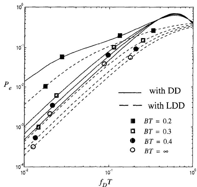
FIGURE 4. The irreducible error rate versus the normalized Doppler for GMSK in a fast Rayleigh fading channel. SNR, CDR, and CIRs are assumed to be infinite.
