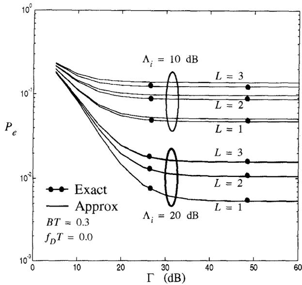
FIGURE 1. The exact and approximate bit error rates of GMSK in a Rayleigh fading environment in the presence of  $L$  cochannel interferers, The detection method is LDD. Infinite CDR is assumed.
