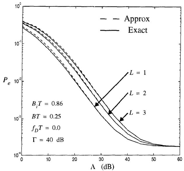
FIGURE 3. The exact and approximate bit error rates of GMSK in a Rayleigh fading environment in the presence of  $L$  cochannel interferers, The detection method is DD. Infinite CDR is assumed. The interferers have random bit-timing offsets with respect to the desired signal.
