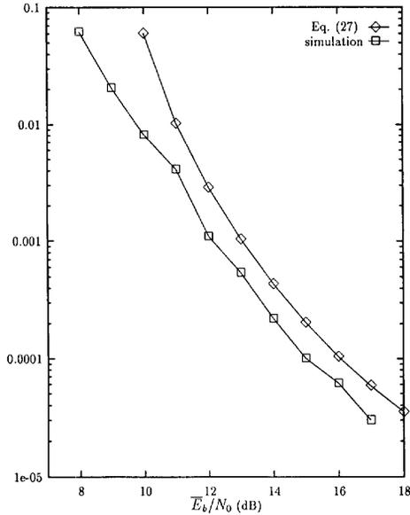
Fig. 8.  $P_b$  versus  $\bar{E}_b/N_0$ . Trellis code in Fig. 3, average shadowed Rician fading, differential detection,  $f_d T_s = 0.05$ .
