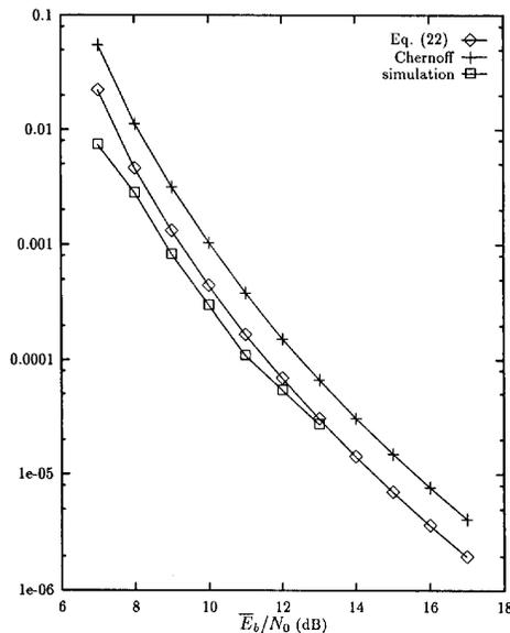
Fig. 7.  $P_b$  versus  $\bar{E}_b/N_0$ . Trellis code in Fig. 3, average shadowed Rician fading, coherent detection.
