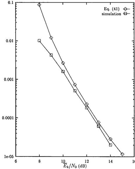
Fig. 12.  $P_b$  versus  $\bar{E}_b/N_0$ . Trellis code in Fig. 3, light shadowed Rician, slow fading, pilot-tone detection,  $f_d T_s = 0.05$ .
