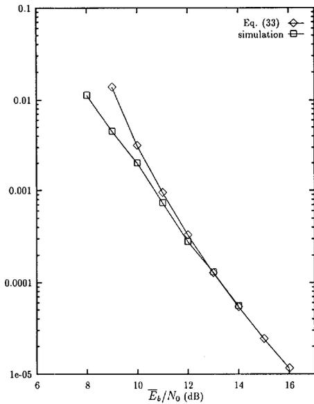
Fig. 9.  $P_b$  versus  $\bar{E}_b/N_0$ . Trellis code in Fig. 3, average shadowed Rician fading pilot-tone detection,  $f_d T_s = 0.05$ .
