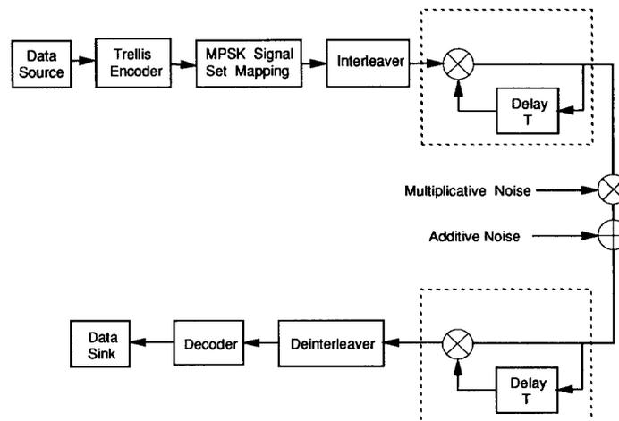
Fig. 1. Baseband system model where  $T_s$  is the symbol period.
