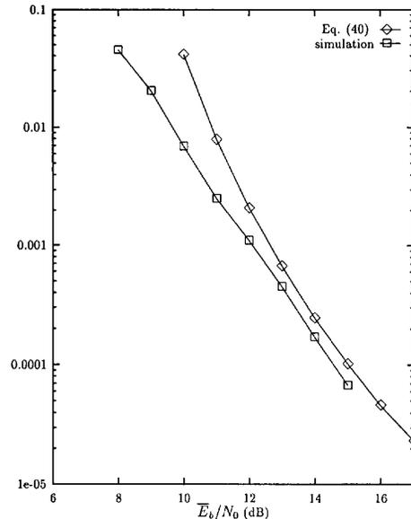
Fig. 11.  $P_b$  versus  $\bar{E}_b/N_0$ . Trellis code in Fig. 3, light shadowed Rician slow fading, differential detection,  $f_d T_s = 0.05$ .
