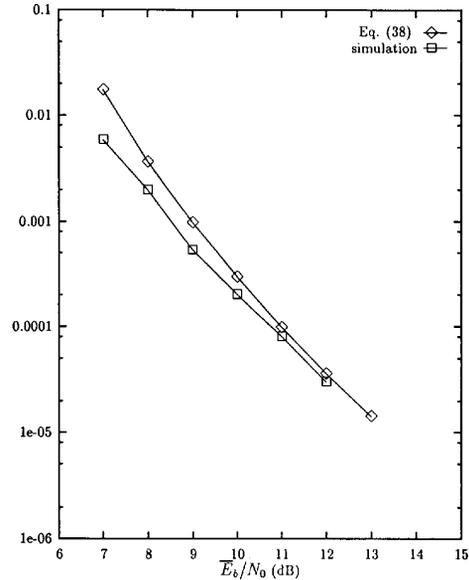
Fig. 10.  $P_b$  versus  $\bar{E}_b/N_0$ . Trellis code in Fig. 3, light shadowed Rician slow fading, coherent detection.
