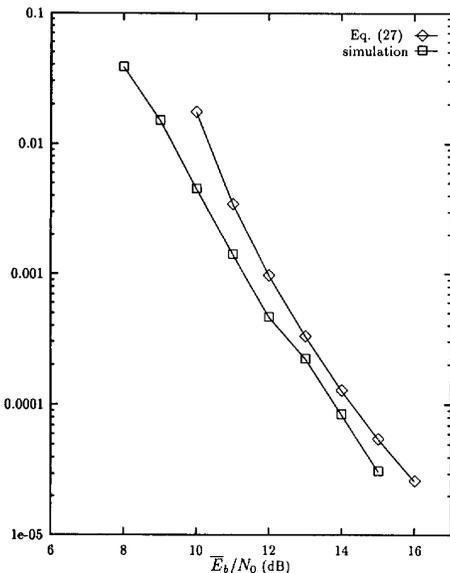
Fig. 5.  $P_b$  versus  $\bar{E}_b/N_0$ . Trellis code in Fig. 3, light shadowed Rician fading, differential detection,  $f_d T_s = 0.05$ .
