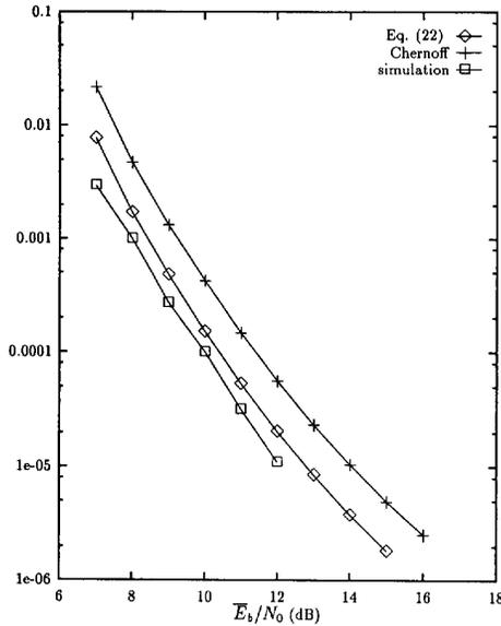
Fig. 4.  $P_b$  versus  $\bar{E}_b/N_0$ . Trellis code in Fig. 3, light shadowed Rician fading, coherent detection.
