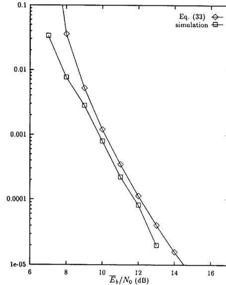
Fig. 6.  $P_b$  versus  $\bar{E}_b/N_0$ . Trellis code in Fig. 3, light shadowed Rician fading, pilot-tone detection,  $f_d T_s = 0.05$ .
