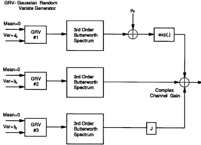
Fig. 2. Shadowed Rician fading simulator.
