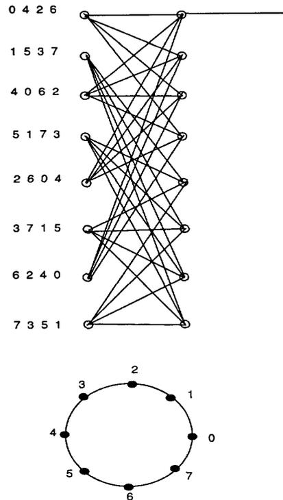
Fig. 3. Trellis diagram for 8-state, 8 PSK TCM scheme [12].
