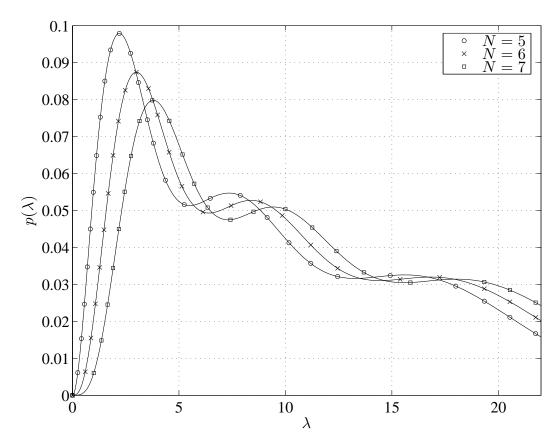
Figure 4.3: The eigenvalue density of uncorrelated noncentral Wishart matrices with M=3,  $\pmb{\gamma}=(2,5,7)^T$  and N=5,6 and 7.
