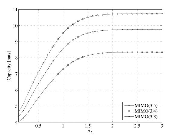
Figure 5.4: The capacity of full–correlated Rayleigh MIMO channels at SNR= $10 {\rm dB}$  with  $\delta=10^{\circ}$ .
