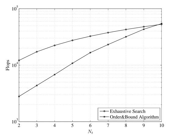
Figure 6.5: Average flops of beamformer selection with the exhaustive search and the order and bound algorithm for MIMO system with  $N_r=5$  receive antennas and  $N_b=7$  bits of feedback versus the number of transmit antennas.
