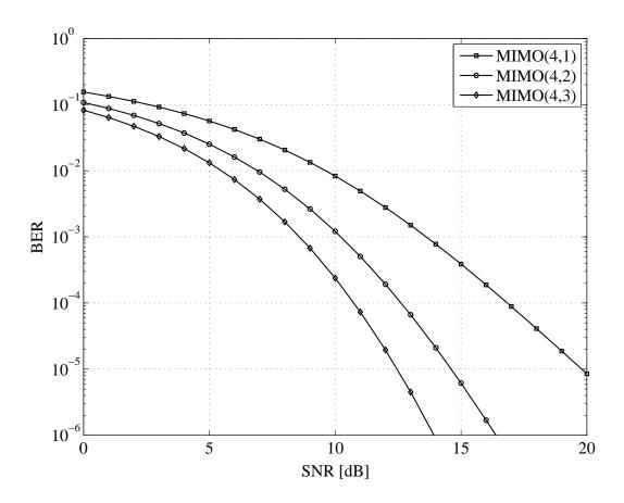
Figure 6.6: BER of optimal transmit beamforming.
