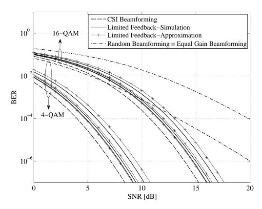
Figure 6.8: BER of MIMO(4,3) system obtained from simulation and closed-form approximation for 4–QAM and 16–QAM signalings. Pair curves from left to right are for  $N_b=7,5$  and 3 feedback bits, respectively.
