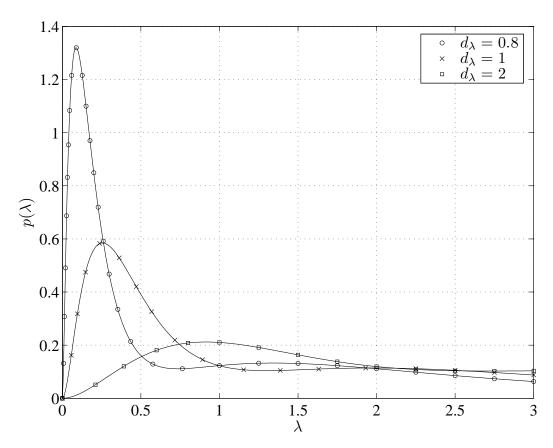
**Figure 4.4:** The eigenvalue density of full-correlated central Wishart matrices with  $N=5,~M=3,~\delta=10^\circ$  and  $d_\lambda=0.8,~1$  and 2. The correlation factors are obtained from (4.19).
