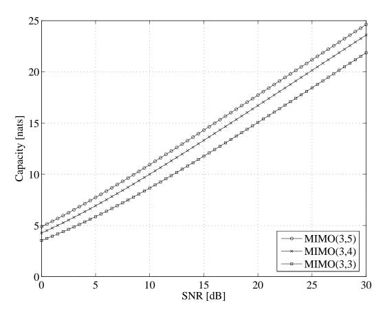
**Figure 5.1:** The capacity of uncorrelated Ricean MIMO channels with eigenvalues  $\gamma = (0.1, 0.3, 0.7)^T$  for the matrix  $\mathbf{G}_0\mathbf{G}_0^*$ .
