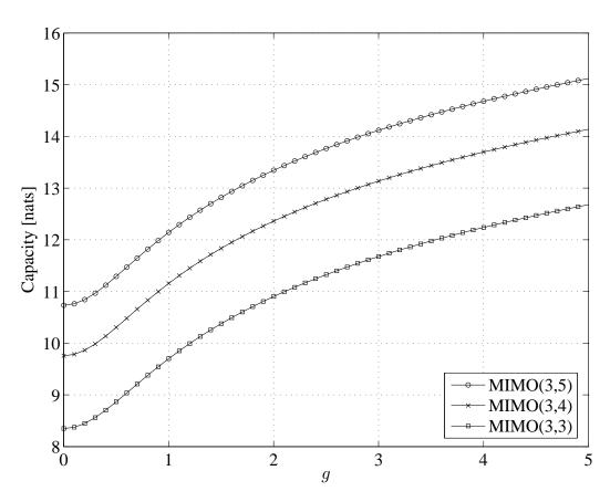
**Figure 5.2:** The capacity of i.i.d. Ricean MIMO channels at SNR=dB with  $\mathcal{CN}(g,1)$  distribution.
