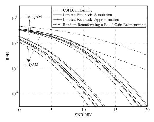
Figure 6.7: BER of MIMO(4,2) system obtained from simulation and closed-form approximation for 4–QAM and 16–QAM signalings. Pair curves from left to right are for  $N_b = 7,5$  and 3 feedback bits, respectively.
