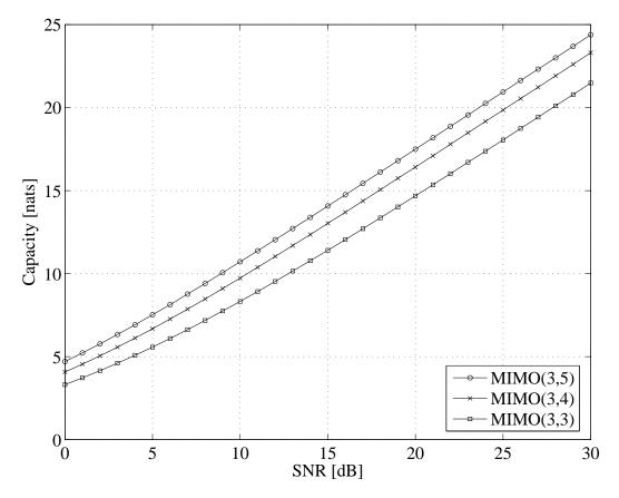
Figure 5.3: The capacity of full–correlated Rayleigh MIMO channels with  $d_{\lambda}=2$  and  $\delta=10^{\circ}.$
