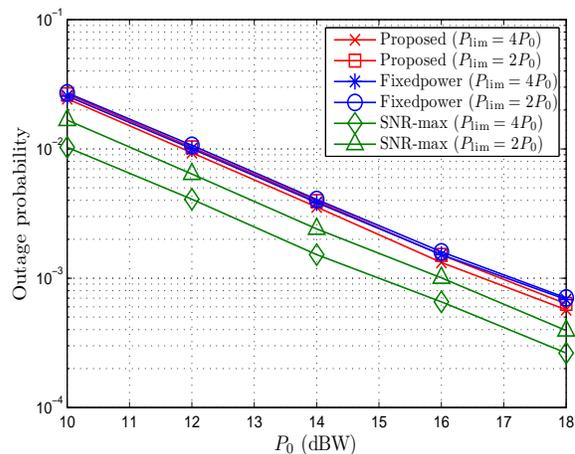
Fig. 6. SNR outage probability versus  $P_0$  for a two-relay network with sum relay power constraint.
