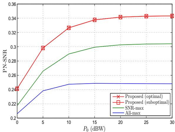
Fig. 7. Average PN-SNR versus  $P_0$  for a two-relay network with separate relay power constraints.
