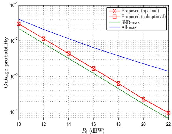
Fig. 8. SNR outage probability versus  $P_0$  for a two-relay network with separate relay power constraints.
