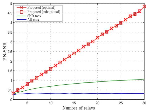
Fig. 9. Average PN-SNR versus number of relays for networks with separate relay power constraints.
