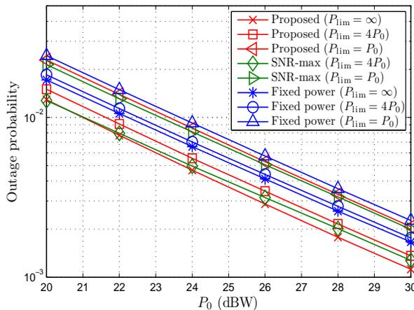
Fig. 4. SNR outage probability versus  $P_0$  for a single-relay network.
