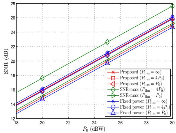
Fig. 3. Average received SNR versus  $P_0$  for a single-relay network.
