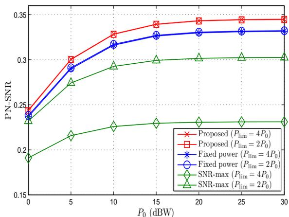
Fig. 5. Average PN-SNR versus  $P_0$  for a two-relay network with sum relay power constraint.
