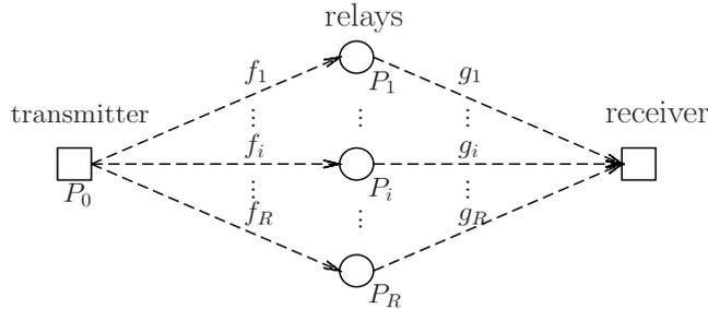
Fig. 1. Multi-relay network.
